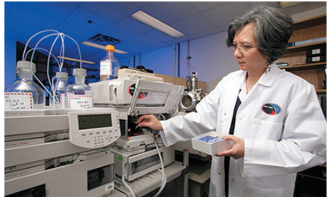
An NRC researcher uses a liquid chromatography-mass spectrometry system to quantify toxins in shellfish samples.
