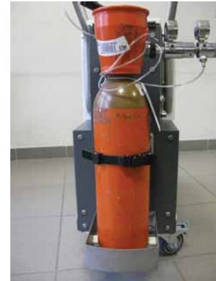
Bottle holder equipped with helium bottle
