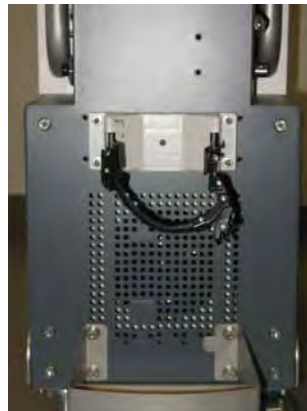
Bottle holder fixed on the leak detector
