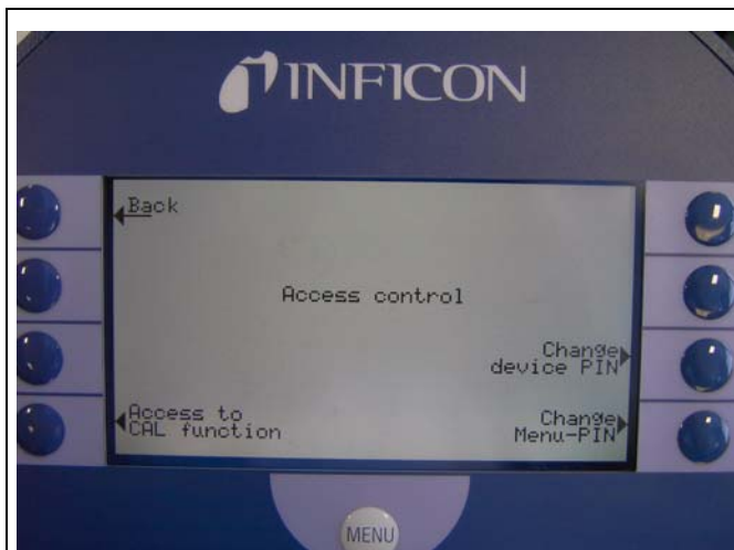
Fig. 4-13: The Access control menu
