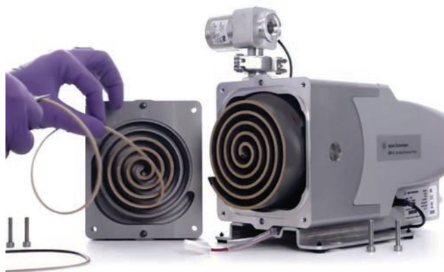
IDP-3 tip seal replacement is fast and easy.
