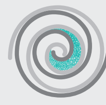
Gas is exhausted at center hub
