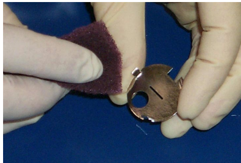
Figure 5-20 Discolored Ground Slit Plate
