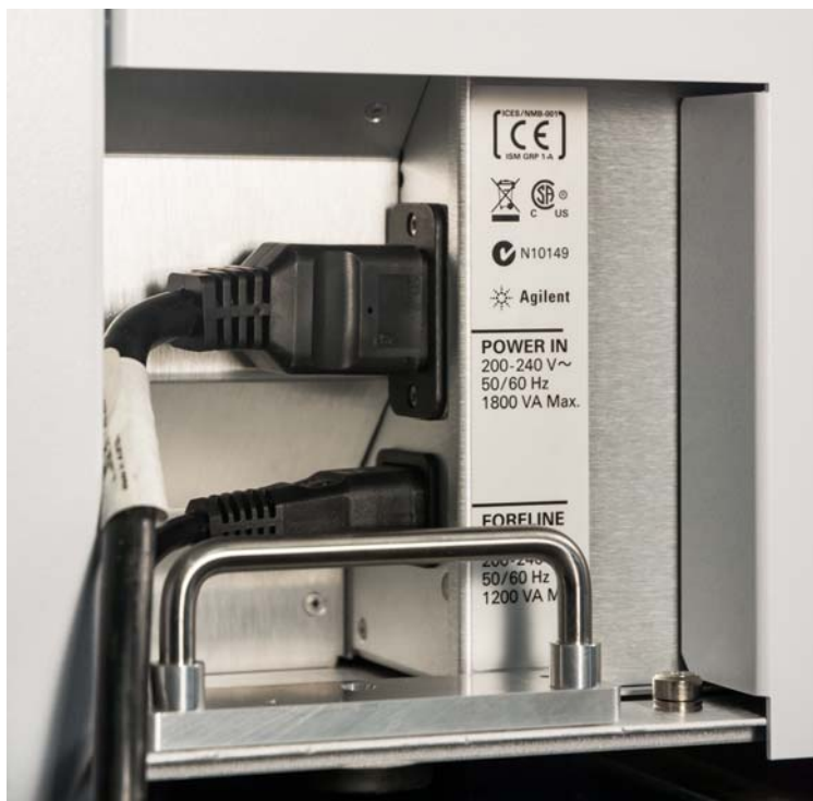
Figure 2 Side panel power supply
