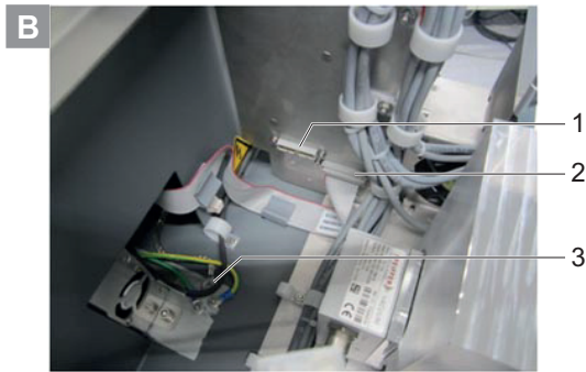
1 J2 connector 2 J1 connector 3 Ground connection
