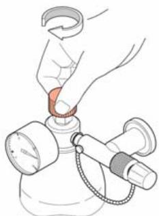
6. Open the vent screw so far, that the pressure drops to the desired pressure. See [Figure 46](#), item 3.
