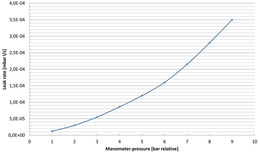
Figure 50 Diagram leak rate/pressure vacuum operation
