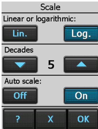
Scaling options of the leak-rate curve and the bar graph:
