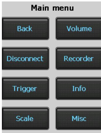
The "Menu" symbol (Figure 9 item 9) can be used to access the main menu for the configuration of the remote control.
