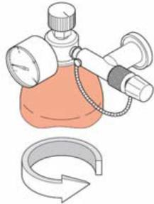
5. Open the test gas supply on the reservoir (the knob turns downwards). See [Figure 46](#), item 2.
