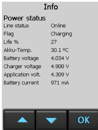
"Info" provides information about the power level of the battery, the wireless connection, etc., and gives information on the current version over 4 pages.
