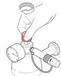
Repeat process steps 6 through 10 twice, so as to ensure that the gas reservoir ahead of the calibrated leak has been exchanged completely. The calibrated leak will now be ready. The desired pressure can be adjusted with the venting screw.
