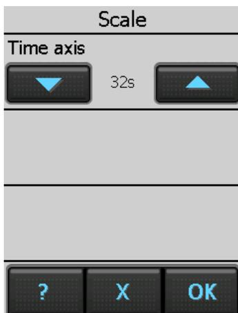
Scaling the time axis of the leak-rate curve:
