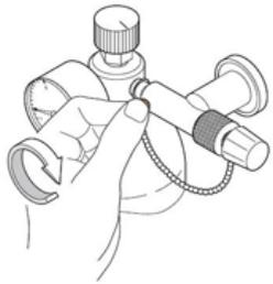
9. Open the test gas supply, so that the pressure reaches the pressure of the test gas cylinder.
