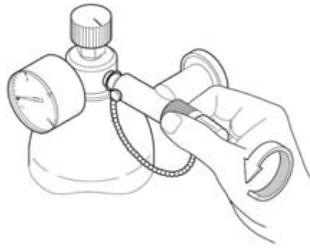
The leak outlet orifice itself is on the face of the sealed-in tubulation which is now visible. The sniffer probe can be inserted into this small orifice. With the screw cap removed the port leaks at the desired reference level.
