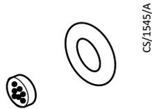
Replace sinter filter and the seal.
