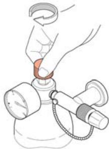
7. Open the vent screw so far that the pressure drops to 0 bar (purge).
