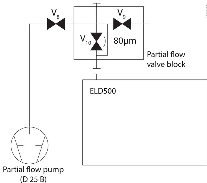
If 3 mbar are decreased, V10 is opened and as described before the GROSS mode is attained with the partial flow pump (V8 and V10 open).
