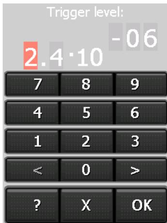
The basic level and exponent of the trigger level of the remote control are set here.
