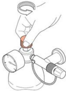
The pressure gauge must now indicate the pressure of the gas bottle.
