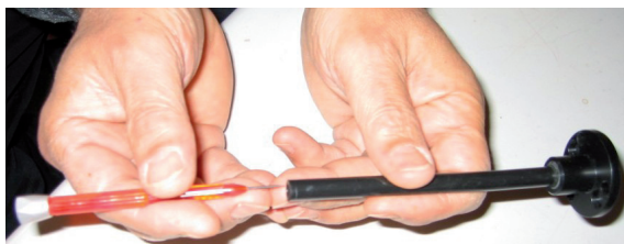
Fig. 6: Press the capillary out of the sniffing tip
