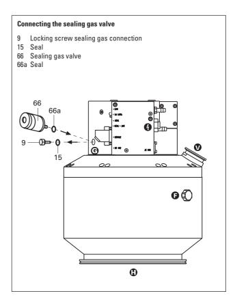
Please refer to Operating Instructions PM 0229 BN for details on installing the sealing gas valve and adjusting the sealing gas flow.
