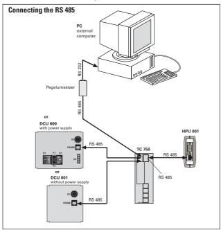
The serial interface is galvanically and safely separated from the maximum supply voltage from the TC 750.
