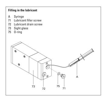
→ Screw back in lubricant filler screw 71 with the 0-ring 75.
