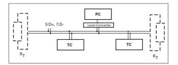
All units connected to the bus must have differing serial interface addresses (parameter 797).
