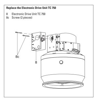
→ Assemble the new Electronic Drive Unit TC 750 (for order number please see Section 10. Spare Parts) on the turbopump and connect again.
