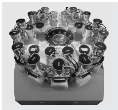
Entire high vacuum equipment of a CD/DVD coating system with TURBOVAC TW 250 S pumps
