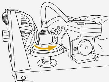
Holding Filter cartridge turn fitting on the top by 1/4 of turn
