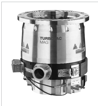
MAG W 1500 CT turbomolecular pump with magnetic rotor suspension and compound stage
