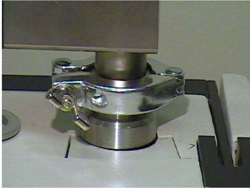
Figure 3-4 Test Port with Connected Device
