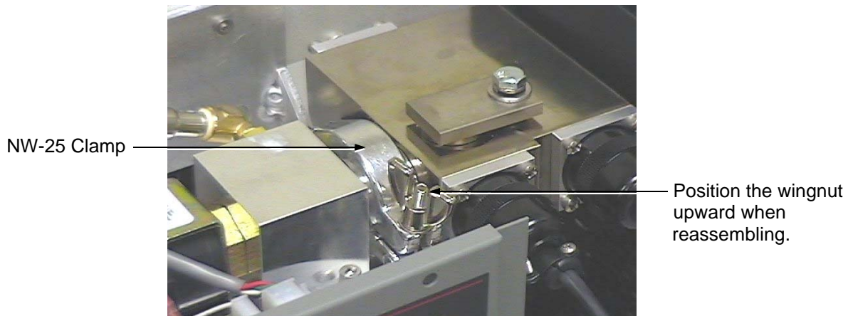
Figure 3-8 Wing Nut and Clamp
