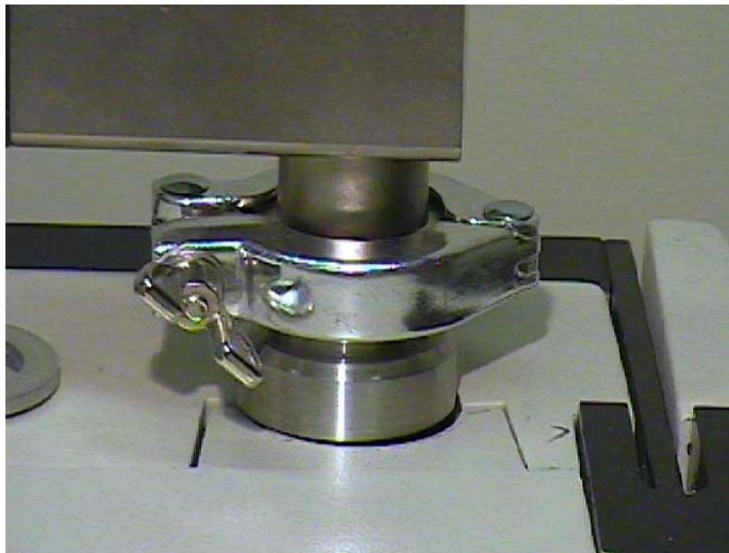
Figure 2-9 Test Port with Connected Device
